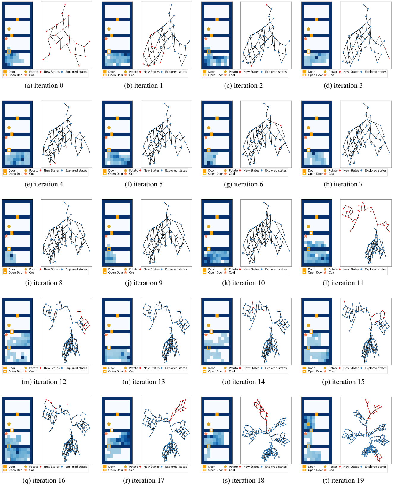
Figure 8: (Eigenoptions Agent) State visitation frequencies and constructed graph per iteration in Minecraft Bake-Rooms
